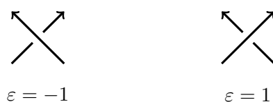
Figure 2.1.2: The two possible types of oriented crossing, referred to as negative and positive crossings respectively.
