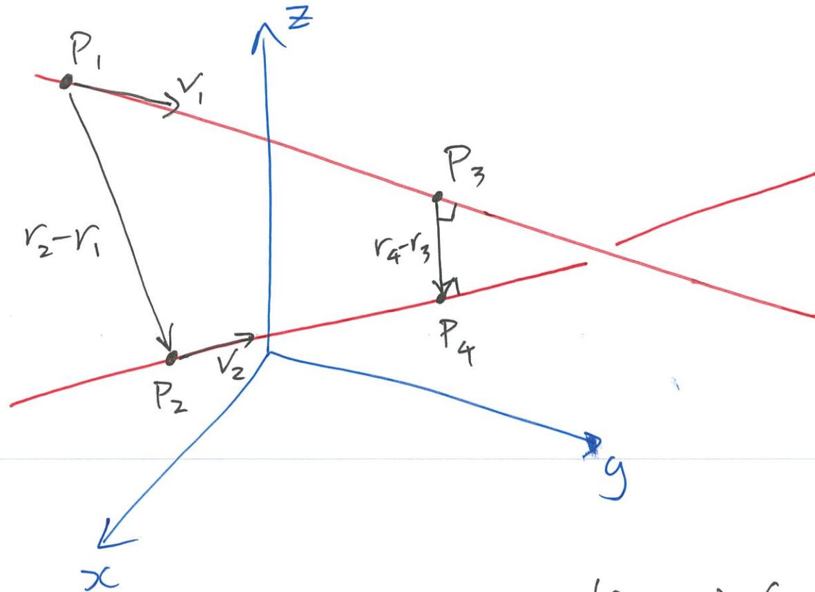
$$d = \|r_4 - r_3\| \text{ which we can rewrite as } d = \frac{|(r_4 - r_3) \cdot (v_1 \times v_2)|}{\|v_1 \times v_2\|}$$
