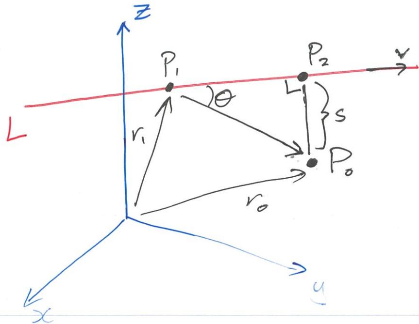
Now  $\|(r_0 - r_1) \times v\| = \|r_0 - r_1\| \|v\| \sin\theta$ , so
